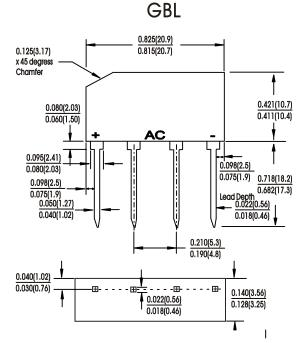
Polarity shown on form side of case: positive lead by beveled cormer Dimensions in inches and (millimeters)
