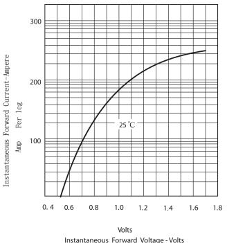
Figure. 2 Forward Derating Curve 250 Average Forward Rectified Current-Ampere Per leg 200 150 100 Single Phase Half Wave 60Hz Resistive or Inductive Load 0 0 50 100 125 150 175 75  $^{\circ}$ C Case Temperature -  $^{\circ}$ C
