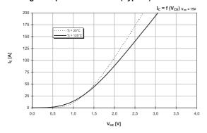
Fig.2 Transfer characteristic (Typical)
