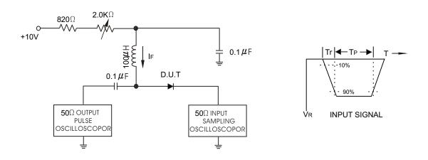
NOTES: 1.A 2.0K Variable resistor for forward current (IF) of 10mA 2.Input pules is adjusted so IR(peak) is equal to 10mA 3.tp" trr
