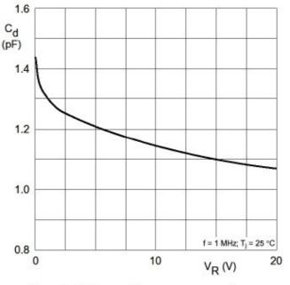
Figure 4. Diode capacitance vs. reverse voltage (Typical values)
