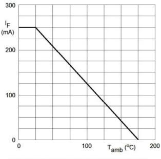
Figure 1. Maximum permissible continuous forward current vs. ambient temperature
