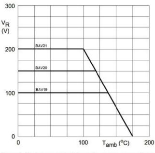
Figure 3. Maximum permissible continuous reverse voltage vs. ambient temperature
