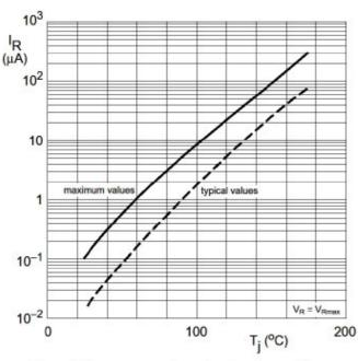
Figure 3. Reverse current vs. junction temperature
