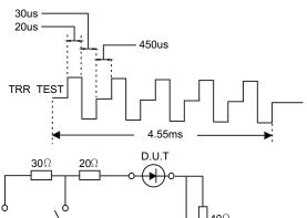
Figure 6 GR1 Test Circuit
