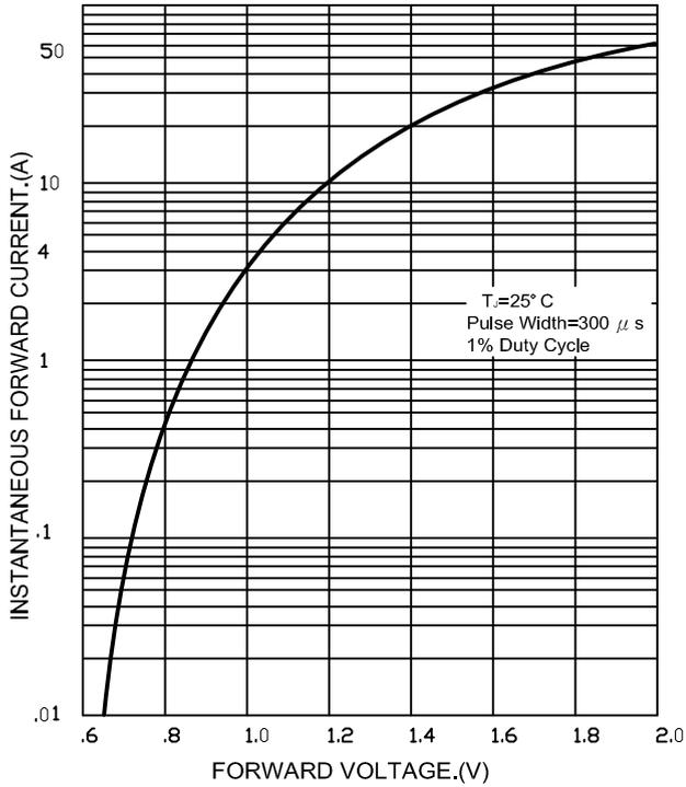
FIG.2 - TYPICAL FORWARD CURRENT DERATING CURVE
