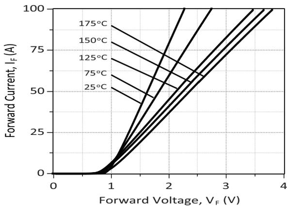
Typical High Current Forward Characteristics (Per diode)
