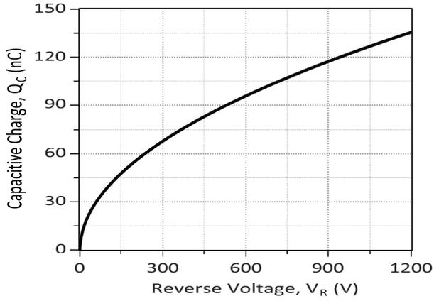
Typical Capacitive Energy vs. Reverse Voltage Characteristics (Per diode)
