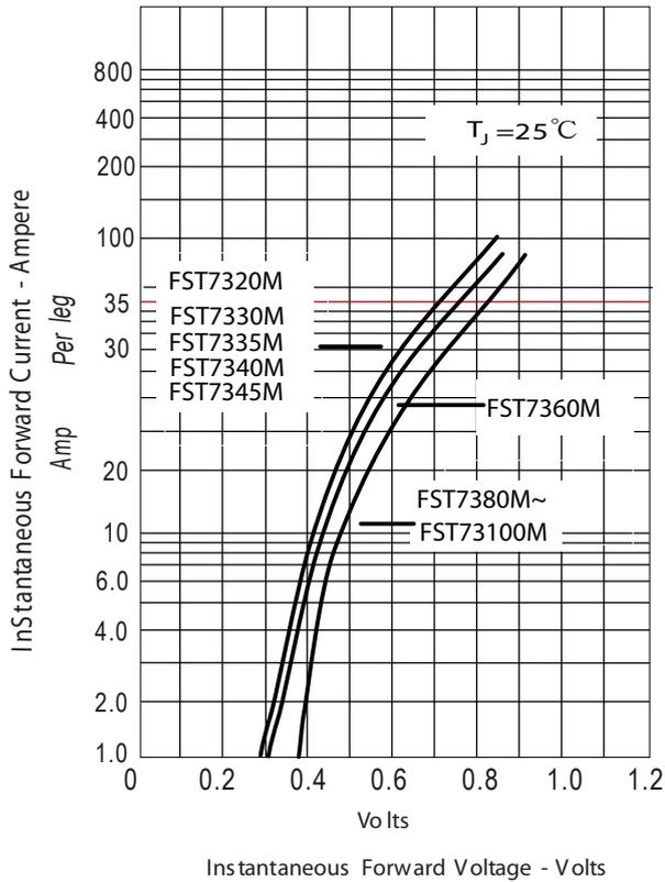
Figure .2- Forward Derating Curve
